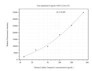
Cytometric bead array standard curve of MP51198-1, Cardiac Troponin I Monoclonal Matched Antibody Pair, PBS Only. Capture antibody: 66376-2-PBS. Detection antibody: 66376-1-PBS. Standard:Ag16758. Range: 12.5-400 ng/mL
