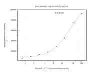
Cytometric bead array standard curve of MP51192-3, FAM114A1 Monoclonal Matched Antibody Pair, PBS Only. Capture antibody: 67926-3-PBS. Detection antibody: 67926-2-PBS. Standard:Ag17289. Range: 0.781-100 ng/mL
