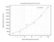
Cytometric bead array standard curve of MP50455-3, OPN, SPP1 Monoclonal Matched Antibody Pair, PBS Only. Capture antibody: 68983-4-PBS. Detection antibody: 68983-5-PBS. Standard:Ag19216. Range: 3.125-100 ng/mL.
