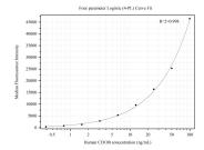
Cytometric bead array standard curve of MP50276-2, CD100 Monoclonal Matched Antibody Pair, PBS Only. Capture antibody: 66582-4-PBS. Detection antibody: 66582-2-PBS. Standard:Ag26461. Range: 0.391-100 ng/mL
