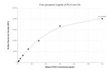
Cytometric bead array standard curve of MP02191-1, CD109 Recombinant Matched Antibody Pair, PBS Only. Capture antibody: 85924-1-PBS. Detection antibody: 85924-3-PBS. Standard: Eg2673. Range: 0.938-120 ng/mL
