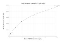
Cytometric bead array standard curve of MP02190-1, TGFBR2 Recombinant Matched Antibody Pair, PBS Only. Capture antibody: 85899-2-PBS. Detection antibody: 98438-1-PBS. Standard: Eg2943. Range: 0.313-20 ng/mL
