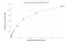
Cytometric bead array standard curve of MP02102-1, PDCD6 Recombinant Matched Antibody Pair, PBS Only. Capture antibody: 85792-4-PBS. Detection antibody: 85792-3-PBS. Standard: Ag2949. Range: 0.781-100 ng/mL
