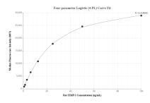
Cytometric bead array standard curve of MP01990-1, RAT TIMP1 Recombinant Matched Antibody Pair, PBS Only. Capture antibody: 85591-2-PBS. Detection antibody: 85591-1-PBS. Standard: Eg3212. Range: 0.781-100 ng/mL
