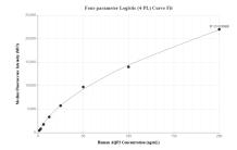
Cytometric bead array standard curve of MP01925-1, AQP2 Recombinant Matched Antibody Pair, PBS Only. Capture antibody: 85402-1-PBS. Detection antibody: 85402-2-PBS. Standard: Ag29931. Range: 1.563-200 ng/mL
