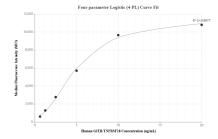
Cytometric bead array standard curve of MP01906-2, GITR/TNFRSF 18 Recombinant Matched Antibody Pair, PBS Only. Capture antibody: 85214-2-PBS. Detection antibody: 85214-1-PBS. Standard: Eg1356. Range: 0.625-20 ng/mL
