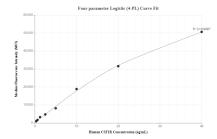
Cytometric bead array standard curve of MP01340-1, CSF1R Recombinant Matched Antibody Pair, PBS Only. Capture antibody: 84477-3-PBS. Detection antibody: 84477-1-PBS. Standard: RP00001. Range: 0.313-40 ng/mL
