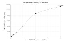
Cytometric bead array standard curve of MP01305-1, TNFRSF17 Recombinant Matched Antibody Pair, PBS Only. Capture antibody: 84419-4-PBS. Detection antibody: 84419-2-PBS. Standard: Eg1812. Range: 0.313-20 ng/mL
