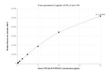
Cytometric bead array standard curve of MP01283-1, MOUSE TWEAK R/TNFRSF12 Recombinant Matched Antibody Pair, PBS Only. Capture antibody: 84423-6-PBS. Detection antibody: 84423-3-PBS. Standard: Eg1838. Range: 0.156-20 ng/mL
