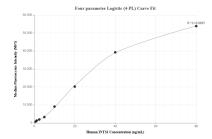
Cytometric bead array standard curve of MP01233-1, INTS1 Recombinant Matched Antibody Pair, PBS Only. Capture antibody: 84339-1-PBS. Detection antibody: 84339-3-PBS. Standard: Ag35428. Range: 0.625-80 ng/mL
