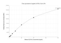
Cytometric bead array standard curve of MP01088-1, CLEC9A Recombinant Matched Antibody Pair, PBS Only. Capture antibody: 84176-4-PBS. Detection antibody: 84176-2-PBS. Standard: Eg1444. Range: 0.625-80 ng/mL
