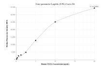
Cytometric bead array standard curve of MP00865-2, VISTA Recombinant Matched Antibody Pair, PBS Only. Capture antibody: 83919-3-PBS. Detection antibody: 83919-2-PBS. Standard: Eg0017. Range: 0.156-20 ng/mL
