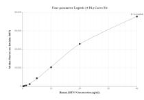
Cytometric bead array standard curve of MP00827-2, LRFN5 Recombinant Matched Antibody Pair, PBS Only. Capture antibody: 83880-4-PBS. Detection antibody: 83880-3-PBS. Standard: Ag22152. Range: 0.313-40 ng/mL
