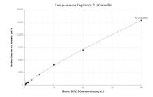
Cytometric bead array standard curve of MP00470-3, FOXC2 Recombinant Matched Antibody Pair, PBS Only. Capture antibody: 83476-1-PBS. Detection antibody: 83476-2-PBS. Standard: Ag33121. Range: 0.313-40 ng/mL
