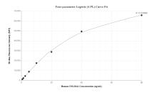
Cytometric bead array standard curve of MP00423-3, COL28A1 Recombinant Matched Antibody Pair, PBS Only. Capture antibody: 83408-4-PBS. Detection antibody: 83408-3-PBS. Standard: Ag21459. Range: 0.625-80 ng/mL
