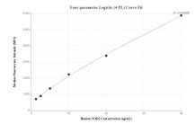
Cytometric bead array standard curve of MP00320-1, NOD2 Recombinant Matched Antibody Pair, PBS Only. Capture antibody: 83281-1-PBS. Detection antibody: 83281-3-PBS. Standard: Ag33771. Range: 1.25-40 ng/mL
