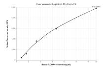
Cytometric bead array standard curve of MP00243-2, SLC 6A9 Recombinant Matched Antibody Pair, PBS Only. Capture antibody: 83150-2-PBS. Detection antibody: 83150-1-PBS. Standard: Ag34437. Range: 1.25-20 ng/mL
