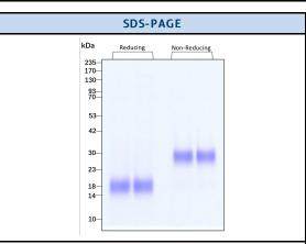
Purity of recombinant human GDNF was determined by SDS- polyacrylamide gel electrophoresis. The protein was resolved in an SDS- polyacrylamide gel in reducing and non-reducing conditions and stained using Coomassie blue.
