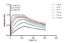
Biolayer interferometry (BLI) kinetic assays of 98226-1-RR against Human C5AR1/CD88 were performed. The affinity constant is 1.56 nM.
