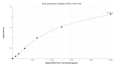
Sandwich ELISA standard curve of MP02892-2, Human DDX4/VASA Recombinant Matched Antibody Pair - PBS only. 87172-4-PBS was coated to a plate as the capture antibody and incubated with serial dilutions of standard Ag0447. 87172-1-PBS was HRP conjugated as the detection antibody. Range: 156-5000 pg/mL.
