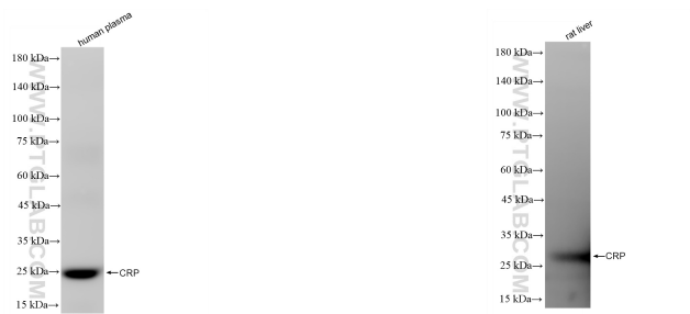
Various lysates were subjected to SDS PAGE followed by western blot with 86912-6-RR (CRP antibody) at dilution of 1:2000 incubated at room temperature for 1.5 hours.
