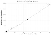
Cytometric bead array standard curve of MP02319-1, Lp-PLA2 Recombinant Matched Antibody Pair, PBS Only. Capture antibody: 86271-2-PBS. Detection antibody: 86271-1-PBS. Standard: Eg3756. Range: 0.781-100 ng/mL
