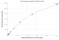
Cytometric bead array standard curve of MP02277-1, Prothrombin/F2 Recombinant Matched Antibody Pair, PBS Only. Capture antibody: 86124-2-PBS. Detection antibody: 86124-1-PBS. Standard: Eg1337. Range: 0.781-100 ng/mL
