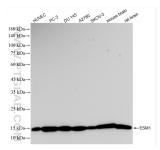
Various lysates were subjected to SDS PAGE followed by western blot with 86027-1-RR (ESM1 antibody) at dilution of 1:5000 incubated at room temperature for 1.5 hours.
