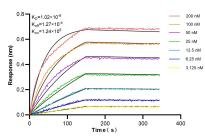
Biolayer interferometry (BLI) kinetic assays of 86009-1-RR against Human RBM47 were performed. The affinity constant is 1.02 nM.
