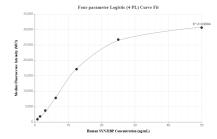
Cytometric bead array standard curve of MP02180-2, SYN12BP Recombinant Matched Antibody Pair, PBS Only. Capture antibody: 85870-2-PBS. Detection antibody: 85870-1-PBS. Standard: Ag8130. Range: 0.781-50 ng/mL
