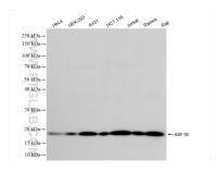
Various lysates were subjected to SDS PAGE followed by western blot with 85848-1-RR (ASF 1B antibody) at dilution of 1:10000 incubated at room temperature for 1.5 hours.
