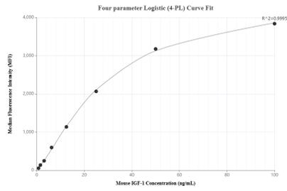
Cytometric bead array standard curve of MP02062-1, MOUSE IGF-1 Recombinant Matched Antibody Pair, PBS Only. Capture antibody: 85644-2-PBS. Detection antibody: 85644-1-PBS. Standard: Eg1939. Range: 0.781-100 ng/mL.
