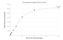
Cytometric bead array standard curve of MP01988-1, MOUSE IL-28A Recombinant Matched Antibody Pair, PBS Only. Capture antibody: 85590-3-PBS. Detection antibody: 85590-2-PBS. Standard: Eg3169. Range: 0.313-40 ng/mL
