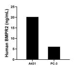
The mean BMPR2 concentration was determined to be 20.20 ng/mL in A431 cell extract based on a 2.70 mg/mL extract load and 6.06 ng/mL in PC-3 cell extract based on a 1.30 mg/mL extract load.
