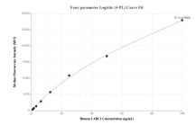
Cytometric bead array standard curve of MP01952-1, CABC1 Recombinant Matched Antibody Pair, PBS Only. Capture antibody: 85431-3-PBS. Detection antibody: 85431-1-PBS. Standard: Ag7612. Range: 0.781-100 ng/mL
