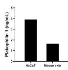
The mean Plakophilin 1 concentration was determined to be 3.9 ng/mL in HaCaT cell extract based on a 1.0 mg/mL extract load and 1.7 ng/mL in mouse skin tissue extract based on a 0.9 mg/mL extract load.
