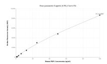
Cytometric bead array standard curve of MP01918-1, PKP1/Plakophilin 1 Recombinant Matched Antibody Pair, PBS Only. Capture antibody: 85217-1-PBS. Detection antibody: 85217-2-PBS. Standard: Ag18153. Range: 0.781-100 ng/mL
