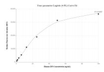
Cytometric bead array standard curve of MP01801-1, ZP3 Recombinant Matched Antibody Pair, PBS Only. Capture antibody: 85084-3-PBS. Detection antibody: 85084-2-PBS. Standard: Ag15791. Range: 0.781-100 ng/mL
