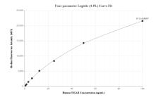
Cytometric bead array standard curve of MP01803-2, TIGAR Recombinant Matched Antibody Pair, PBS Only. Capture antibody: 85052-4-PBS. Detection antibody: 85052-3-PBS. Standard: Ag17532. Range: 0.781-100 ng/mL
