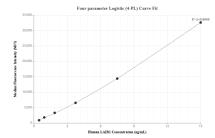
Cytometric bead array standard curve of MP01466-2, LAIR1 Recombinant Matched Antibody Pair, PBS Only. Capture antibody: 84677-3-PBS. Detection antibody: 84677-2-PBS. Standard: Eg2329. Range: 0.469-15 ng/mL
