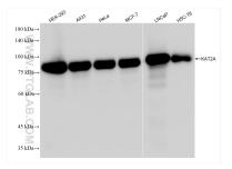
Various lysates were subjected to SDS PAGE followed by western blot with 84669-2-RR (KAT2A/GCN5 antibody) at dilution of 1:5000 incubated at room temperature for 1.5 hours.
