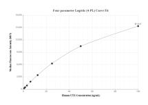
Cytometric bead array standard curve of MP01453-2, UTX Recombinant Matched Antibody Pair, PBS Only. Capture antibody: 84614-1-PBS. Detection antibody: 84614-2-PBS. Standard: Ag36754. Range: 0.781-100 ng/mL
