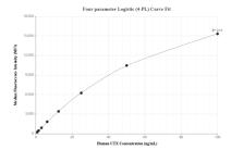
Cytometric bead array standard curve of MP01453-2, UTX Recombinant Matched Antibody Pair, PBS Only. Capture antibody: 84614-1-PBS. Detection antibody: 84614-2-PBS. Standard: Ag36754. Range: 0.781-100 ng/mL.
