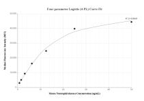
Cytometric bead array standard curve of MP01355-1, MOUSE Neutrophil elastase Recombinant Matched Antibody Pair, PBS Only. Capture antibody: 84473-2-PBS. Detection antibody: 84473-4-PBS. Standard: Eg2126. Range: 0.781-50 ng/mL
