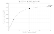
Cytometric bead array standard curve of MP01248-1, MOUSE CD28 Recombinant Matched Antibody Pair, PBS Only. Capture antibody: 84368-5-PBS. Detection antibody: 84368-3-PBS. Standard: Eg1408. Range: 0.313-40 ng/mL
