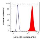
1x10^6 PC-3 cells were intracellularly stained with 0.25 ug ALKBH3 Recombinant antibody (84314-2-RR, Clone:241650F10) and APC-Conjugated Goat Anti-Rabbit 1gG(H+L)(red), or 0.25 ug Isotype Control (blue). Cells were fixed with 4% PFA and permeabilized with Flow Cytometry Perm Buffer (PF00011-C).
