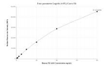
Cytometric bead array standard curve of MP00979-3, TICAM2 Recombinant Matched Antibody Pair, PBS Only. Capture antibody: 84064-2-PBS. Detection antibody: 84064-1-PBS. Standard: Ag17325. Range: 0.625-80 ng/mL
