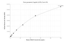
Cytometric bead array standard curve of MP00555-3, TRIM15 Recombinant Matched Antibody Pair, PBS Only. Capture antibody: 83582-2-PBS. Detection antibody: 83582-4-PBS. Standard: Ag4533. Range: 0.78-100 ng/mL
