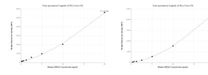
Cytometric bead array standard curve of MP00542-2, GPR161 Recombinant Matched Antibody Pair, PBS Only. Capture antibody: 83557-4-PBS. Detection antibody: 83557-3-PBS. Standard: Ag30998. Range: 0.156- 20 ng/mL Cytometric bead array standard curve of MP00542-3, GPR161 Recombinant Matched Antibody Pair, PBS Only. Capture antibody: 83557-4-PBS. Detection antibody: 83557-1-PBS. Standard: Ag30998. Range: 0.313- 20 ng/mL
