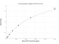
Sandwich ELISA standard curve of MP00528-2, Human TIGIT Recombinant Matched Antibody Pair -PBS only. 83545-1-PBS was coated to a plate as the capture antibody and incubated with serial dilutions of standard Eg0749. 83545-4-PBS was HRP conjugated as the detection antibody. Range: 78.1-5000 pg/mL
