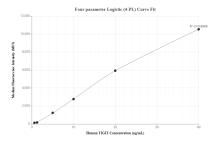
Cytometric bead array standard curve of MP00528-2, TIGIT Recombinant Matched Antibody Pair, PBS Only. Capture antibody: 83545-1-PBS. Detection antibody: 83545-4-PBS. Standard: Eg0749. Range: 0.625-40 ng/mL
