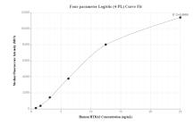
Cytometric bead array standard curve of MP00491-2, HTRA2 Recombinant Matched Antibody Pair, PBS Only. Capture antibody: 83492-5-PBS. Detection antibody: 83492-1-PBS. Standard: Ag8455. Range: 0.781-25 ng/mL
